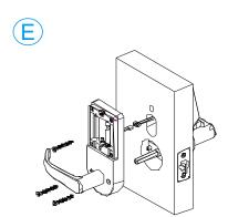
Put the plastic baseboard on the other side of the door, and then connect the cable with the back panel. Install the back panel on the door, and then fasten the lock with the screws.
