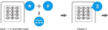
1.Input \* + #, and then input the master password to log in the system
