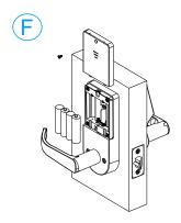
Install the batteries and check the lock.
