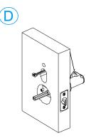
Put the plastic baseboard on the door, and then install the front panel. Check the cable and make it go through the door.
