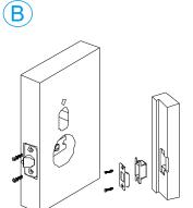
Install the latch and fasten it with screws. Install the strike box and strike and fasten them with screws.
