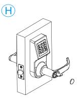
Take out the cylinder cover and try to use the key to unlock and check the installation.
